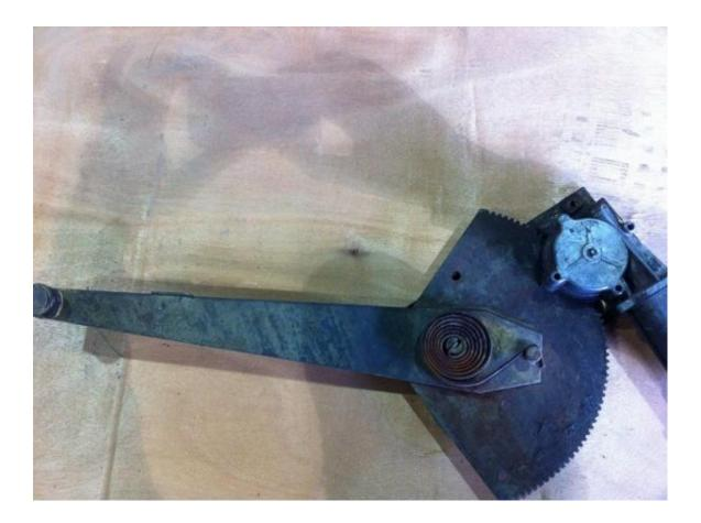
**\*\*\*\*\*WORD OF CAUTION\*\*\*\*** I highlighted in yellow the hole where I placed a screwdriver so the recoil spring wouldn't remove my fingers when I unbolted the motor.
