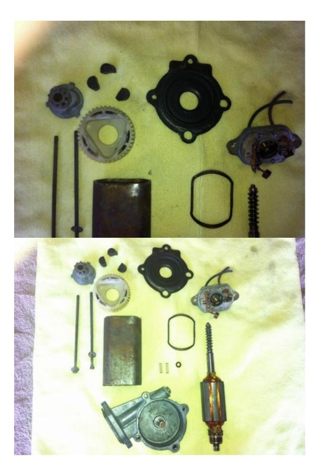
I cleaned everything up using a combination of degreaser, wire wheel, bead blaster, Dremel rotary tool and old fashion scrubbing.
