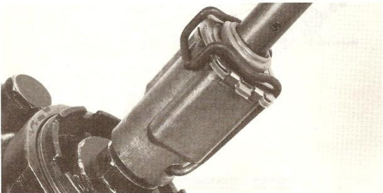
FIGURE 7. STEERING COUPLING CLAMP IN POSITION
