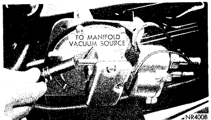
Fig. 6—Removing or Installing Servo Hose
