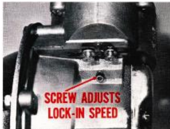
Fig. 26—Screw adjusts accuracy of lock-in speed
