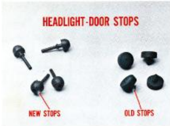
Fig. 39—New bumpers reduce door operating noise
