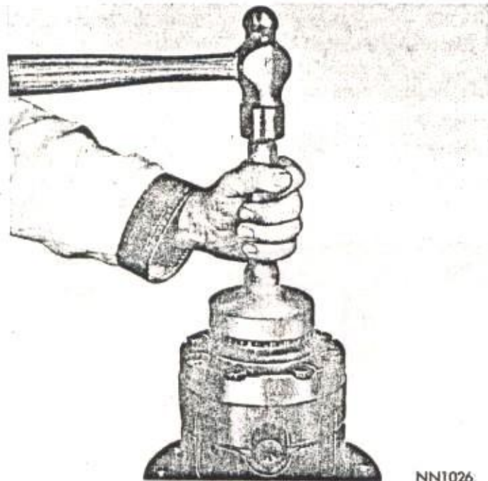
Fig. 9—Installing Differential Bearing Cones
