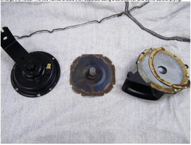
The horn half is cast aluminum. The electrical side is steel. The diaphragm is spring-steel, and the whole thing is put together with paper gaskets and no sealer. No wonder they get corroded over time! I made some new gaskets with some construction paper my kids had lying around. Use whatever color you have!
