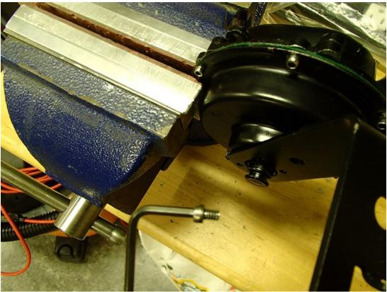
I used a vice (gently) and vice-grips with rubber hose over the ends on the other side to gently squeeze the two sides together, then ran in the 4 screws. The two nearest the horn opening are fake, as I
