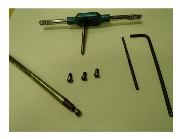
You can see I made a fixture out of a piece of rod to hold the screws while I ground them down a bit to make them look more like the proper rivets. They were  $6-32 \times 1/4$ " and were a bit too long, so I took a few threads off the length as well.
