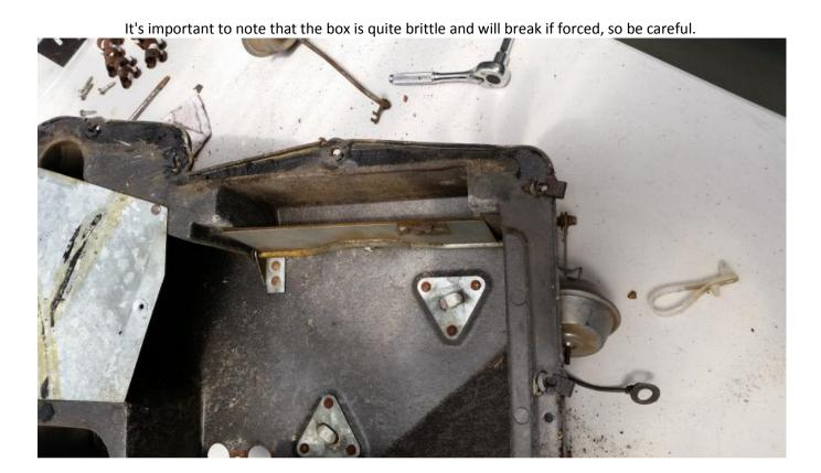
Step 4: Remove heater core and AC evaporator (if equipped). There are a series of screws holding this in place. When removed, bag and tag them.
