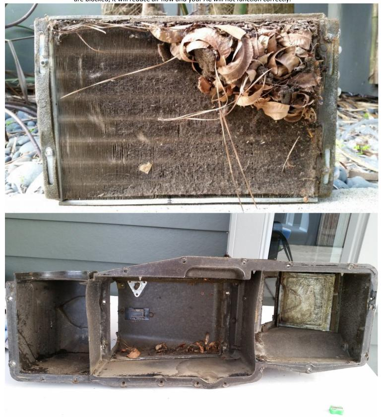
Step 5: Strip all remaining items like actuators and brackets from the housing. Bag and tag them. Then thoroughly clean it. I used a couple of methods. First I pressure washed it (not heavy) and then to remove the stubborn gasket material, a blade and a light wire wheel. This box is brittle so go easy. This resto requires patience.
