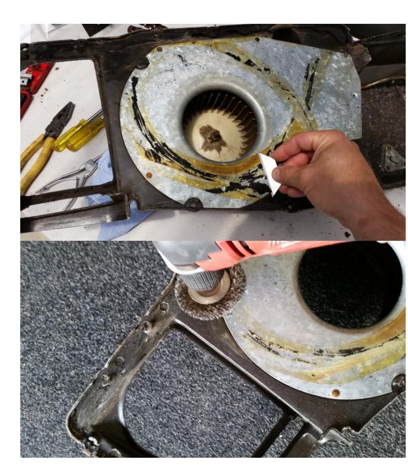
Step 6: Remove all the sticky residue from the internal doors which originally used to be for holding the old seals. I used Peel Off and it worked great. It is a citrus based product. Check out your local Home Depot for some glue solvent. After removal, use denatured alcohol to make sure you get it clean and free from oils and wax etc. It's essential for good adhesion for your foam. Apply all foam as per instructions supplied with your rebuild kit.
