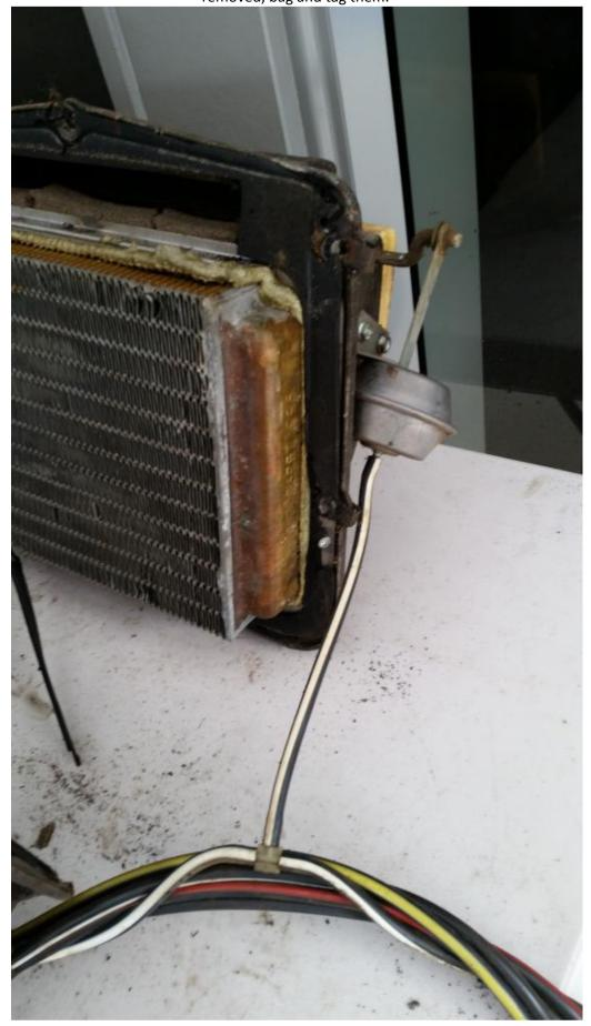
The inside of your box will undoubtedly look similar to this. Give it a good cleaning with a vacuum cleaner with brush attachment, compressed air dust gun and pressure wash gently to ensure that it is back to new condition. If these fins are blocked, it will reduce air flow and your AC will not function correctly.
