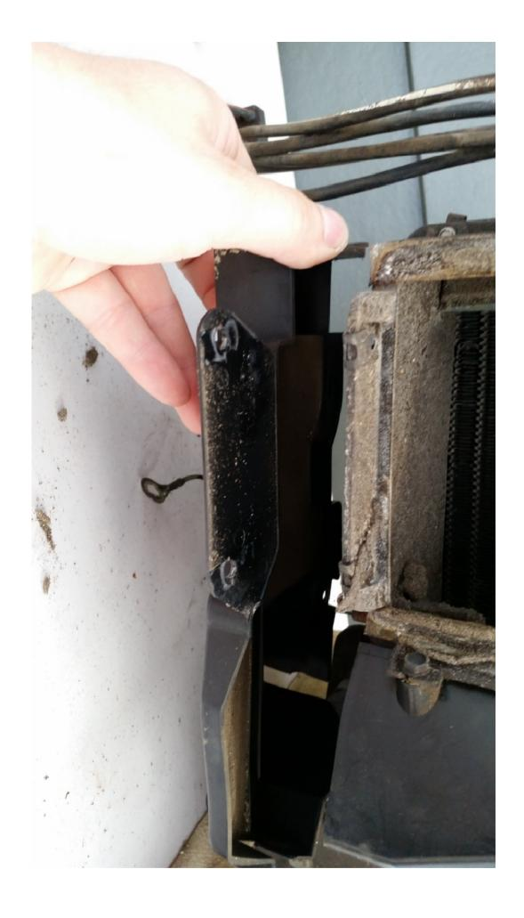
Step 3: Remove the spring clips and gently pry open the two halves. They will be quite stuck as there is a gasket between the mating surfaces. They have been together for 40 plus years so it's no surprise.
