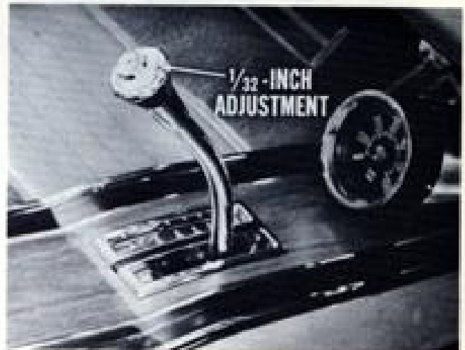
Fig. 20—Console shift release button adjustment
