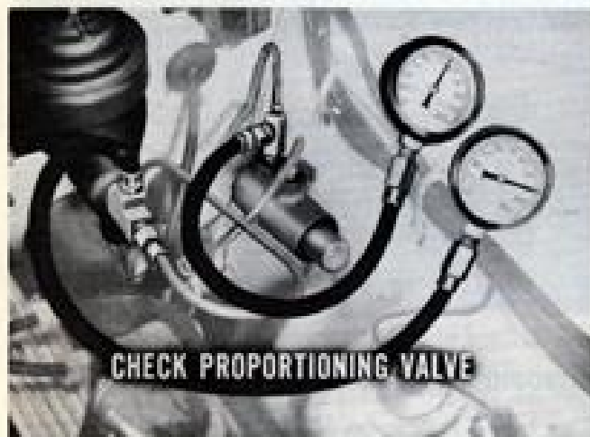
Fig. 24—Proportioning valve must reduce pressure
