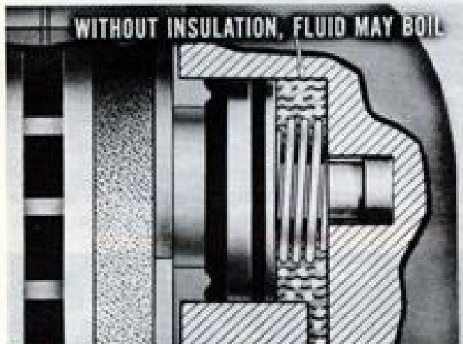
Fig. 26—Insulator keeps the piston cool
