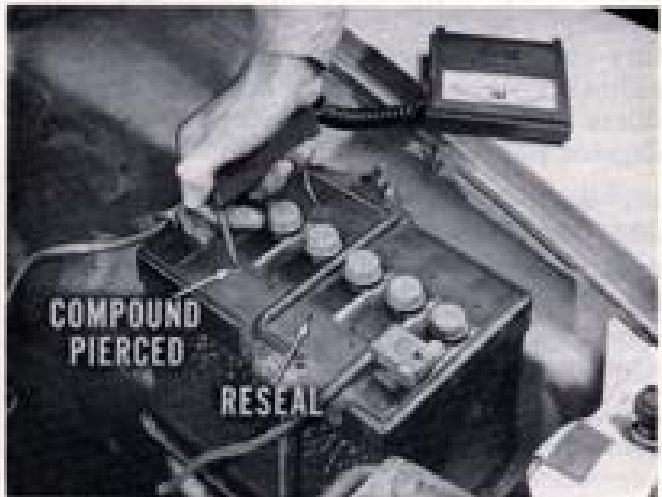
Fig. 10 - Reseal against surface leakage
