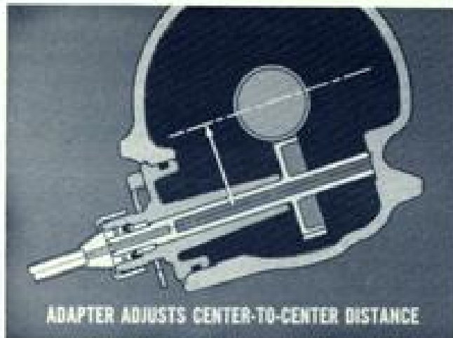
Fig. 23—The new adapter adjusts for different pinion diameters
