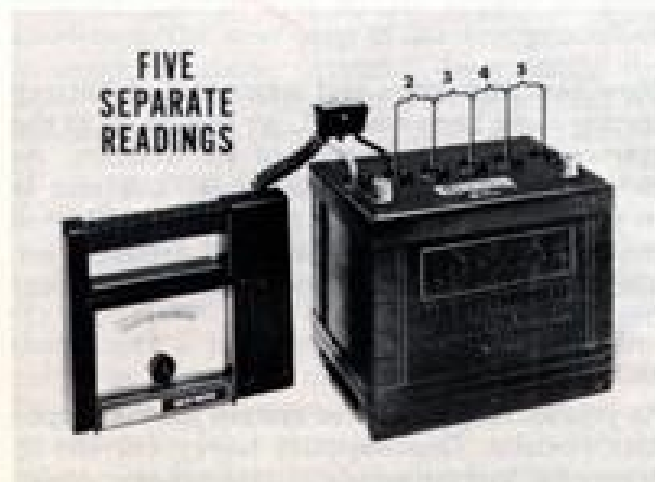
Fig. 12 — Place test probes in adjacent cells
