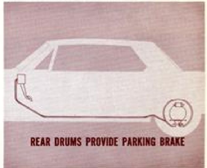
Fig. 3—Drum brakes for parking
