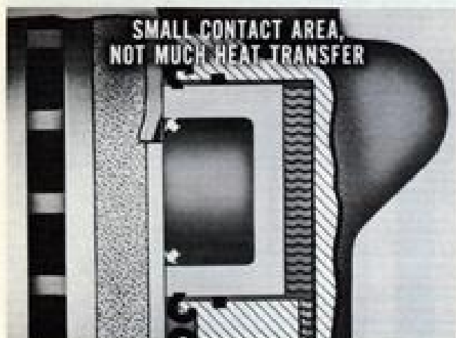
Fig. 11—Hollow pistons don't conduct heat
