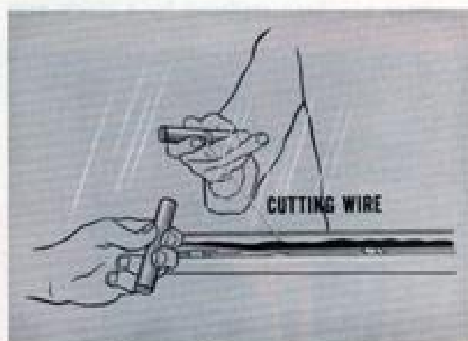
Fig. 5—Steel music wire used to cut caulking
