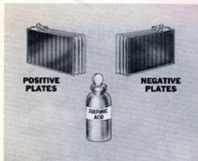
Fig. 2 — Positive and negative plates plus electrolyte
