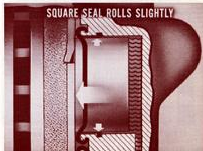
Fig. 9—The piston rolls the seal
