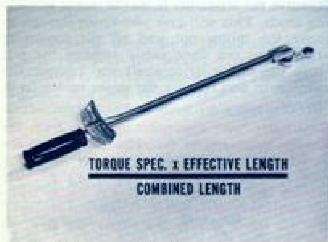
Fig. 12—You must calculate the correct torque reading
