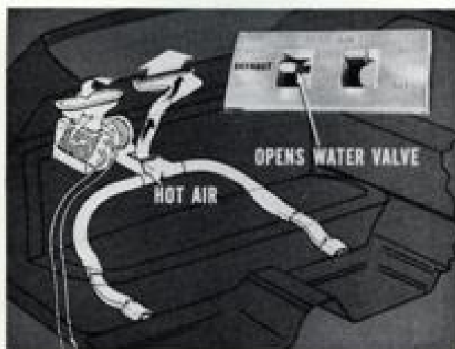
Fig. 30—Rear-seat heater, defrosting air flow
