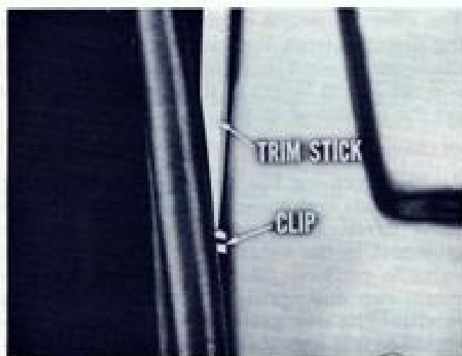
Fig. 10—Trimstick releases weatherstrip clip
