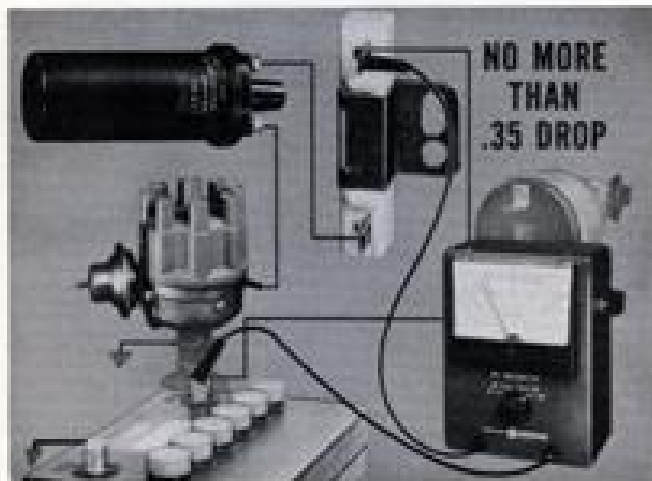
Fig. 25 — Check run-circuit voltage drop
