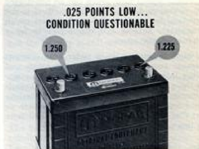
Fig. 8 — Cell reading differences indicate trouble
