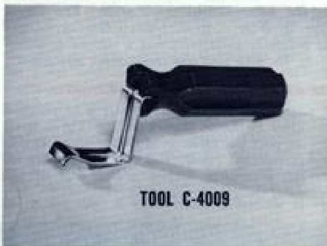
Fig. 8—New windshield and rear window removing tool
