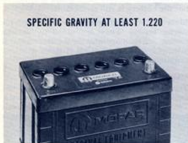
Fig. 14 — Load test needs \frac{3}{4} charge or better
