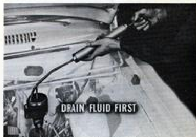
Fig. 22—Make room for fluid in the calipers
