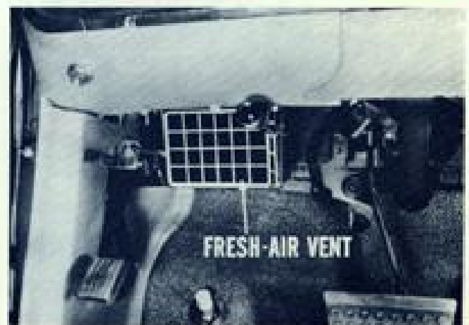
Fig. 25—Belvedere-Coronet vent for driver's side
