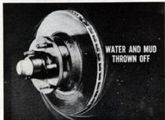
Fig. 1—Discs are self-cleaning
