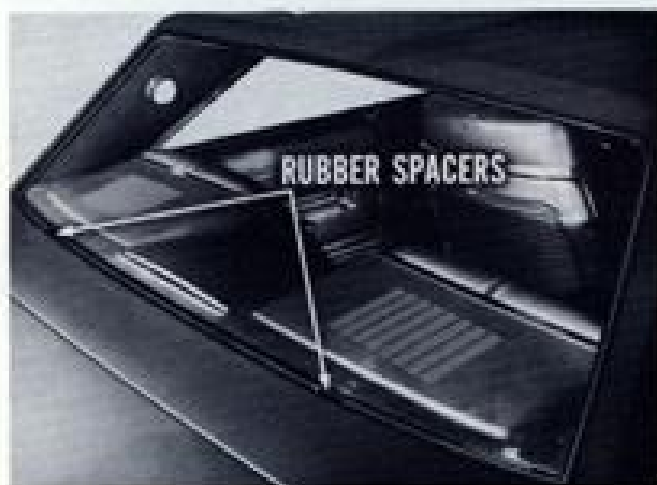
Fig. 6—Rubber spacers support the glass
