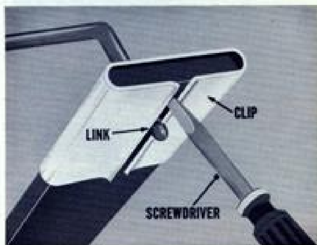
Fig. 11—Screwdriver releases link retaining clip
