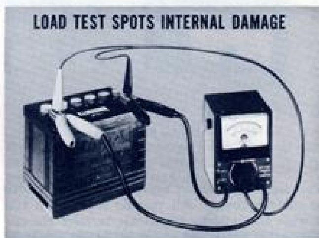
Fig. 15 — Below 9.5 volts calls for replacement
