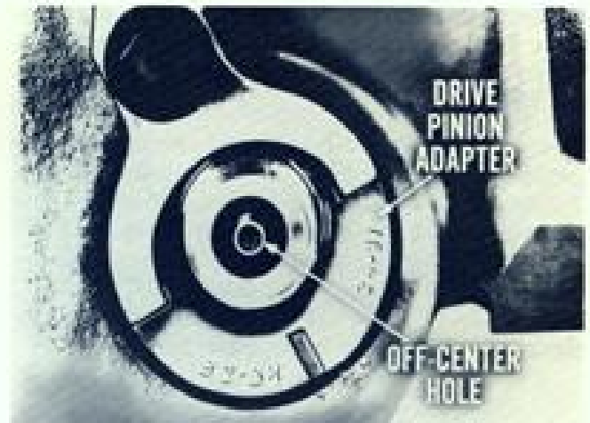
Fig. 24—Adjustable pinion adapter
