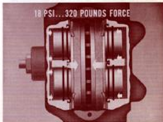
Fig. 8—Residual pressure would cause drag
