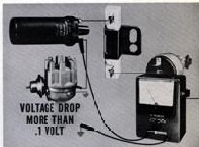
Fig. 27 — Voltage drop indicates distributor resistance
