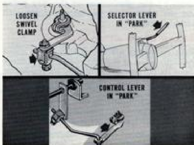
Fig. 18—Torqueflite control rod adjustment
