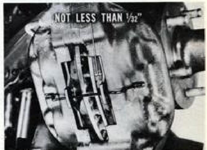
Fig. 29—Maximum lining wear
