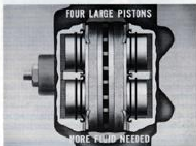
Fig. 6—Higher fluid requirements
