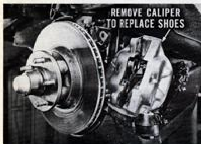
Fig. 30—It's not necessary to open hydraulic lines
